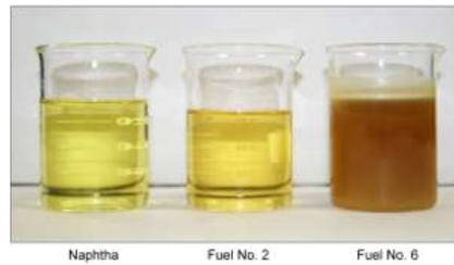
Figure 18: Range of fuel products of P2O process. Source: <http://www.plastic2oil.com/site/fuel-products>.
