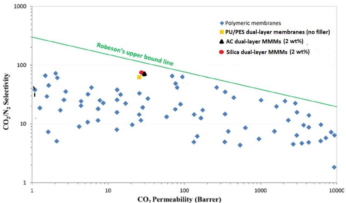
Fig 4.5. PU/PES dual-layer membranes in the 2008 Robeson diagram
