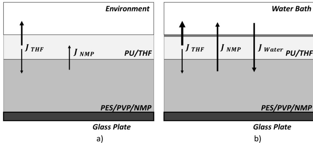
Fig 3.3. Membrane formation: expected fluxes in the co-casting process during a) exposure to environment, b) immersion in water bath.
