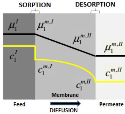
Fig 2.4. Transport through dense membranes (adapted from Silva, 2016).
