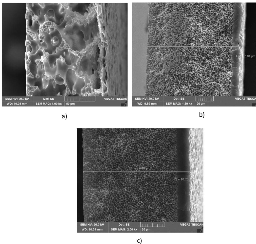
Fig 3.2. Cross-sectional images of the dual-layer membranes prepared using different water bath temperatures: a) 25 °C, b) 50 °C, c) 75 °C.
