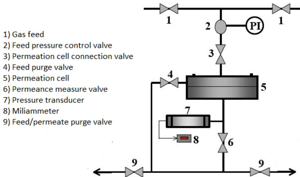
Figure A.1. Diagram of the permeation system for pure gases
