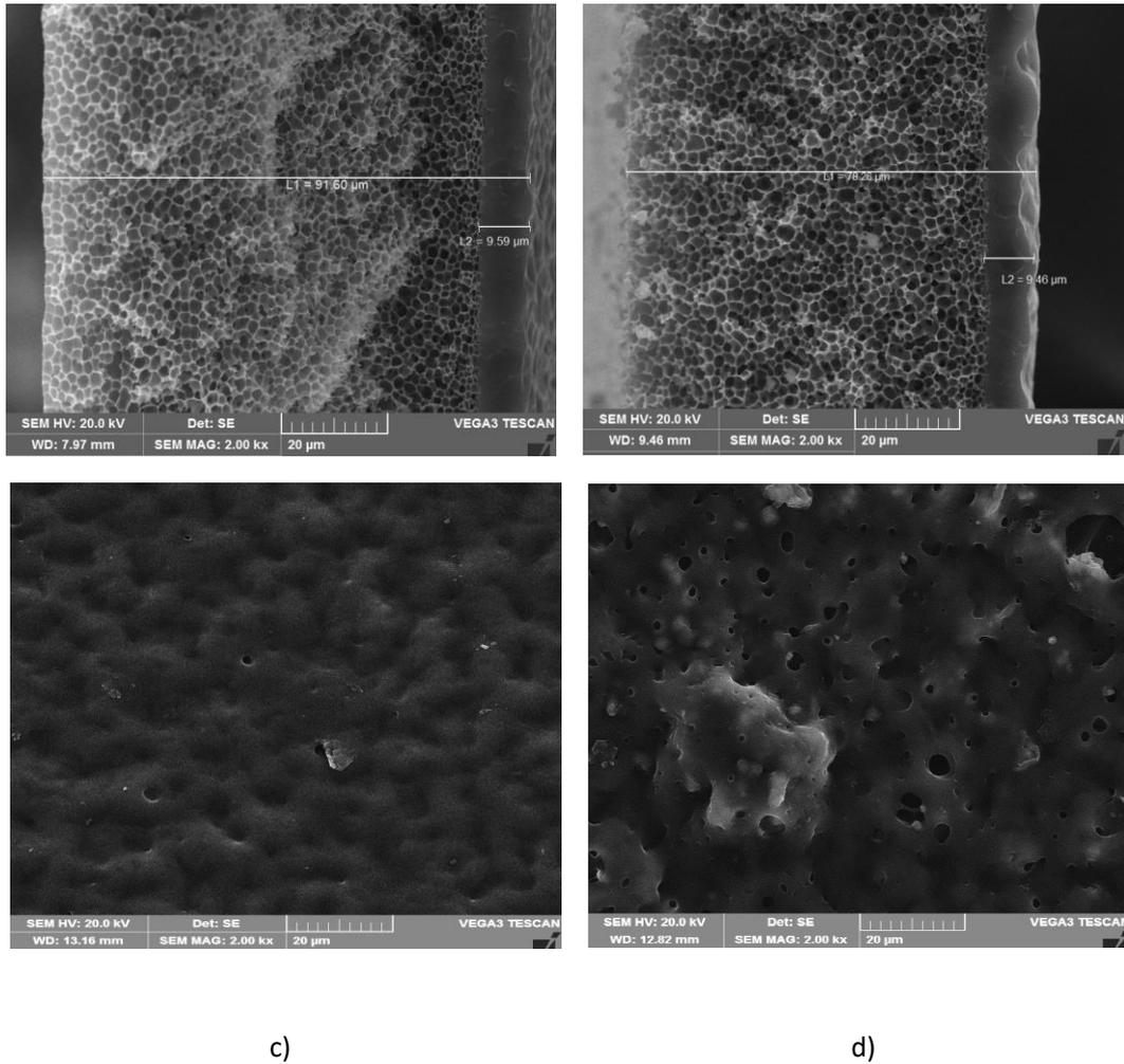
Fig 4.2. Cross-sectional and surface images of the composite membranes with different AC composition in the dense layer a) 0, b) 1, c) 2, d) 5. (AC %wt)
