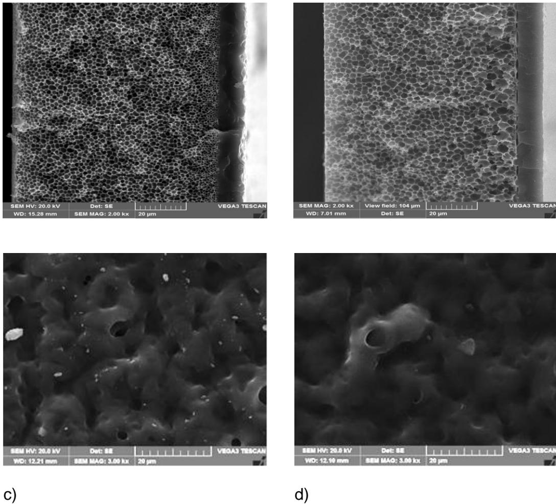
Fig 4.3. Cross-sectional and surface images of the composite membranes prepared using different silica compositions a) 0, b) 1, c) 2, d) 5. (% wt):
