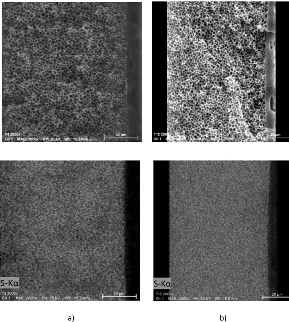
Fig 3.5. Cross-sectional images (Energy Dispersive X-Ray Spectroscopy – EDS) of the dual-layer membranes prepared with different exposure time: a) 15 s, b) 30 s.
