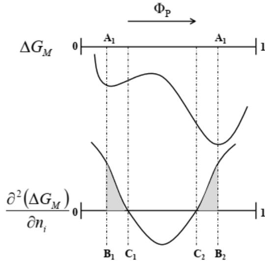
Figure 2.6. Upper: Representation of the variation in free energy of mixing as a function of polymer concentration  $\phi$ , Lower: Representation of the second derivative curve for the free energy of mixing for the composition of the polymeric solution. Source: Carvalho (2005).
