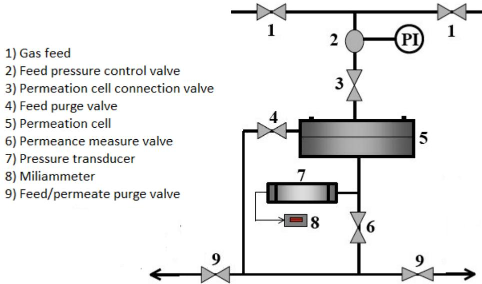
Figure 4.1. Diagram of the permeation system for pure gases
