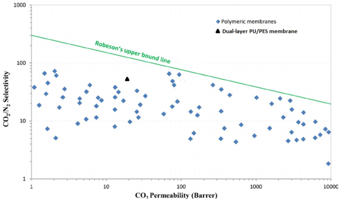
Fig 3.6. PU/PES dual-layer membranes in the 2008 Robeson diagram.
