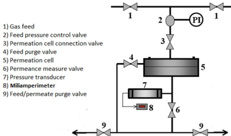
Figure 3.1. Diagram of the permeation system for pure gases
