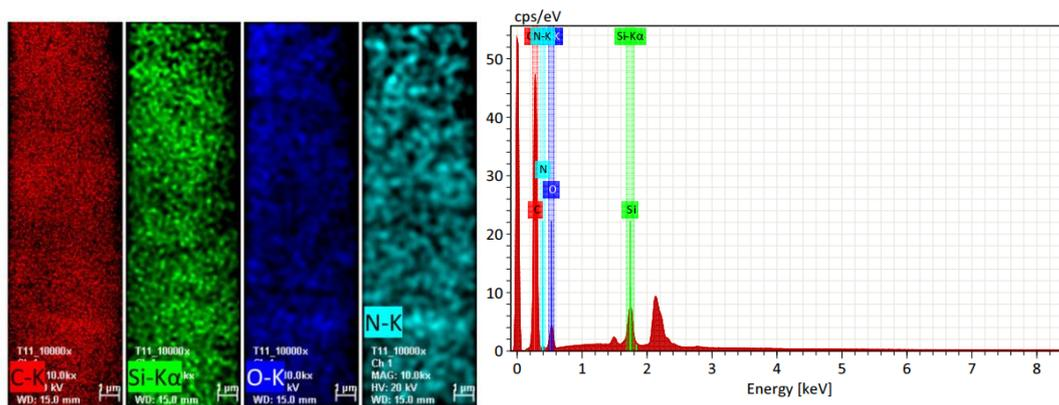
Fig 4.4. EDS images and spectrum for the dense layer with silica particles of PU/PES membranes.
