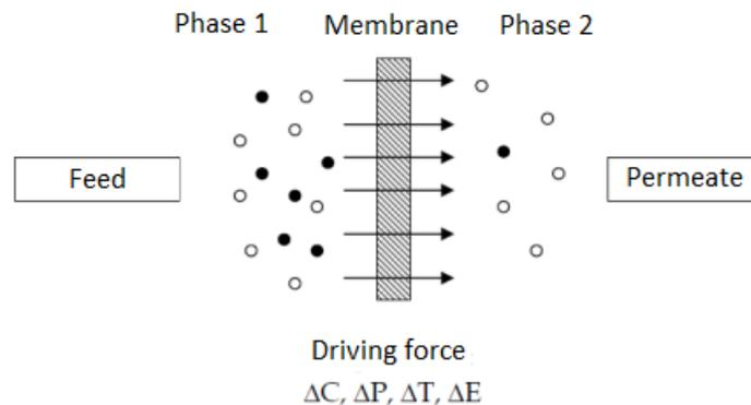
Figure 2.1. Membrane process (adapted from MULDER, 2000).
