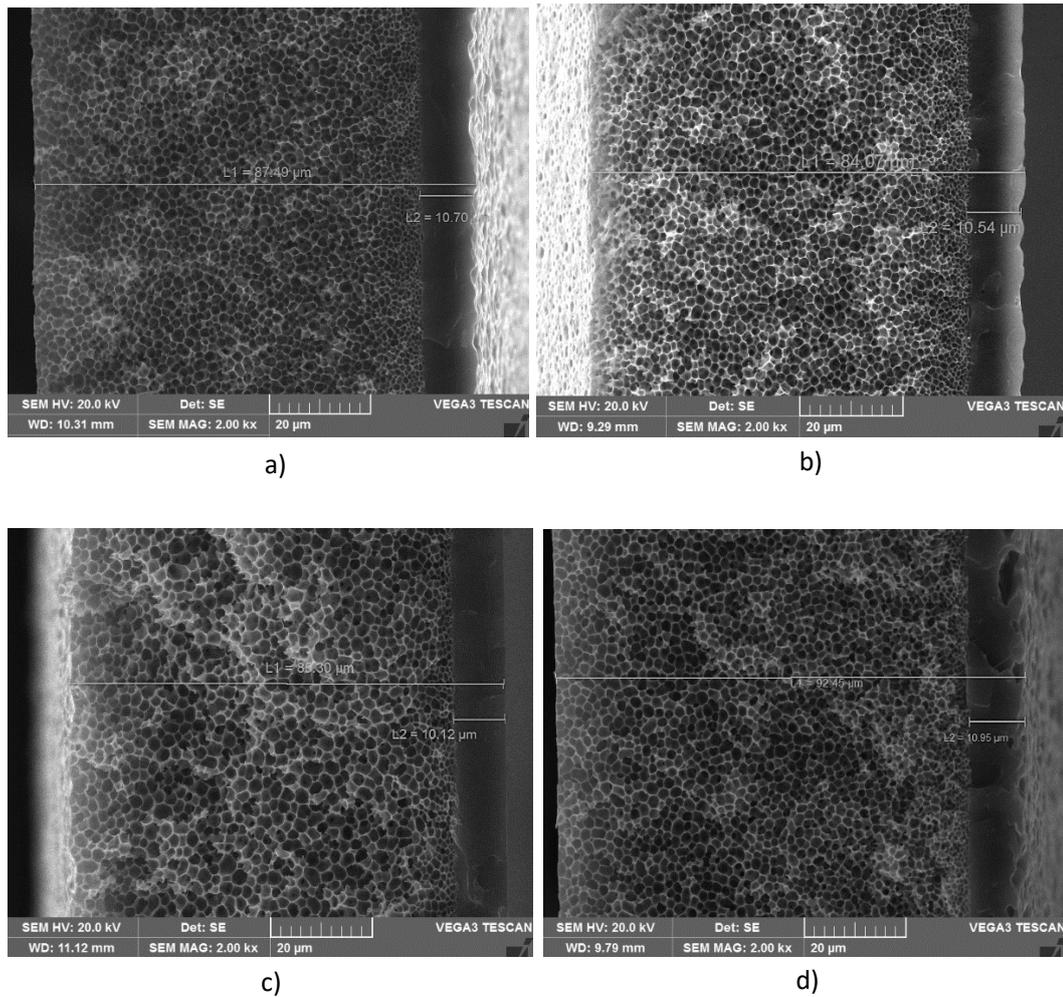
Fig 3.4. Cross-sectional images of the dual-layer membranes prepared using different exposure times: a) No evaporation b) 5 s c) 15 s d) 30 s.
