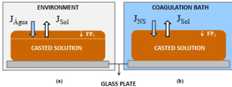
Figure 2.5. Casting process (a) during exposition to environment, (b) after immersion into the coagulation bath.
