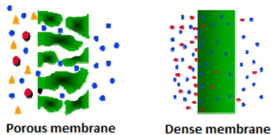
Fig 2.3. Gas permeation through porous and dense membranes adapted from HABERT *et al.*, 2006).
