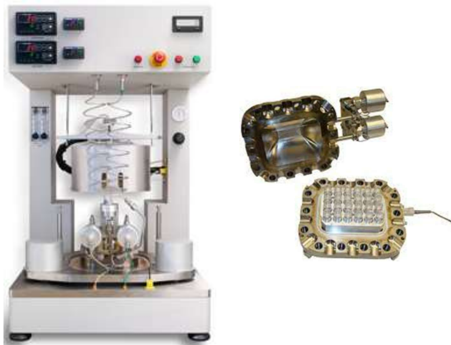
Figure 3.1. Screening Pressure Reactor (SPR).
