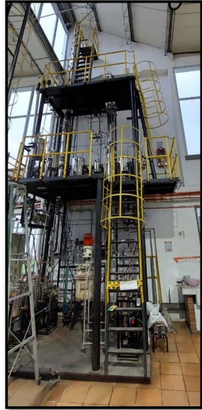
Figure 3.35: Representation of the multistage reactive distillation column.
