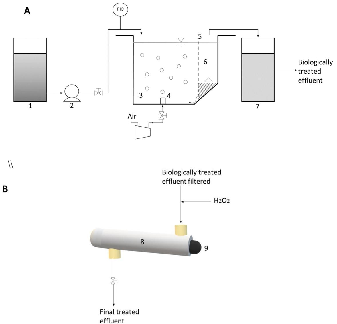
\*(1) feed tank, (2) pump, (3) activated sludge aeration chamber (volume 2.2L), (4) air diffuser, (5) adjustable baffle, (6) settling chamber (volume 0.8L), (7) treated effluent tank, (FIC) flow indicator and control, (8) Stainless Steel 316 vessel with working volume of 1.0L. Chamber dimensions: height 145mm, depth 153mm, length 485mm, manufacturer NovaCura, (9) 20 W UV lamp model Germilamp code 10543,  $6.8\text{W}\cdot\text{m}^{-2}$  fluence with monochromatic emission at 254.0 nm.
