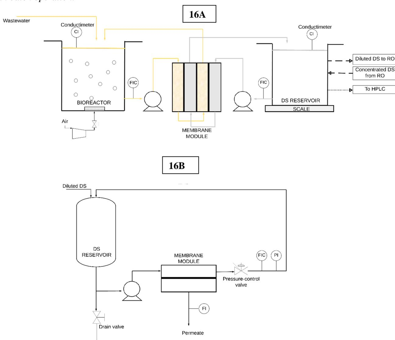
\*Dashed lines in 1A mean whenever DS conductivity dropped below the setpoint, DS was sent to RO for reconcentration and meanwhile it was replaced by previously reconcentrated DS. Dotted line in 1A means that in some predetermined periods of
