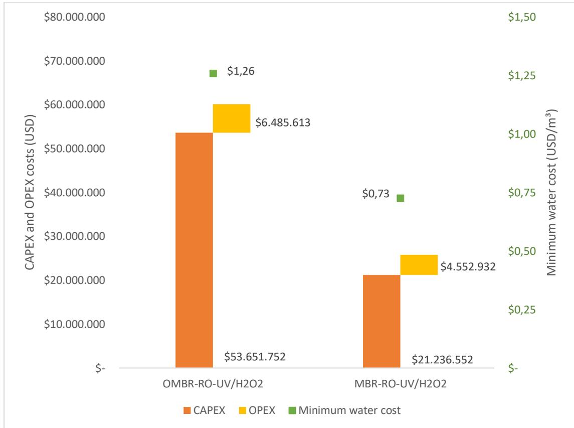
\*Minimum water cost calculated based on plant water capacity of 24,000 m<sup>3</sup>.day<sup>-1</sup> and zero NPV throughout the 20-year lifetime of the project for a interest rate of 5.68% per year.
