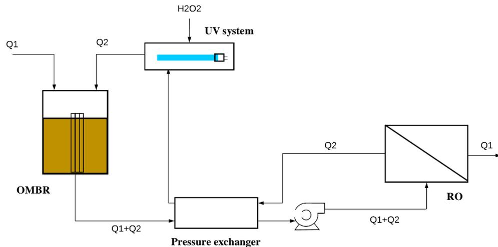
Concentrated DS (Q2) is diluted by the extraction of water from the mixed liquor through the FO membrane, Q1, which corresponds to the flow of influent wastewater. Q2 is considered to be a solution of K<sub>4</sub>P<sub>2</sub>O<sub>7</sub> with osmotic pressure of 11 bar (in sensitivity analysis osmotic pressures ranging from 9 to 25 bar were also assessed). Q1+Q2, corresponding to the diluted DS, is fed to the RO for recover. RO permeate is the reuse water and corresponds to Q1.
