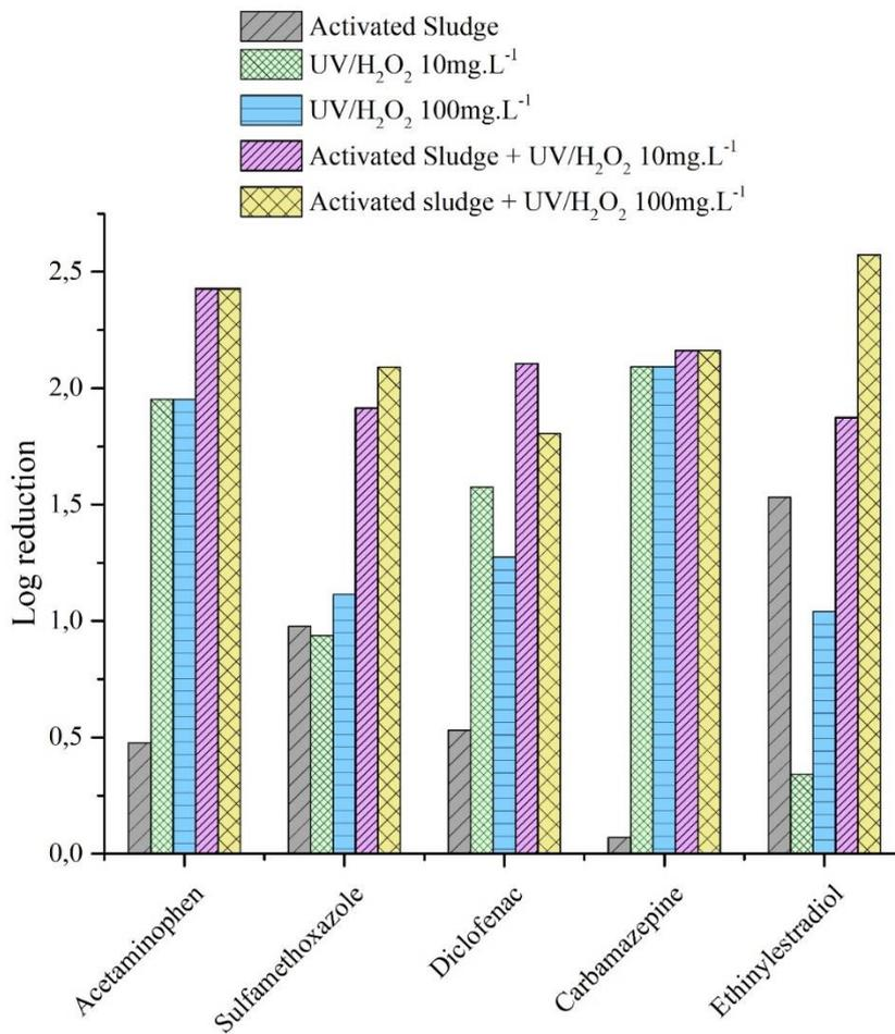
\*The reductions informed in this figure were calculated considering the values at the entrance and at the exit of each process, which were: for AS, synthetic feed and biologically treated effluent; for UV/H<sub>2</sub>O<sub>2</sub> only, biologically treated effluent before and after UV/H<sub>2</sub>O<sub>2</sub>; and for AS+UV/H<sub>2</sub>O<sub>2</sub>, synthetic feed and biologically treated effluent after UV/H<sub>2</sub>O<sub>2</sub>.
