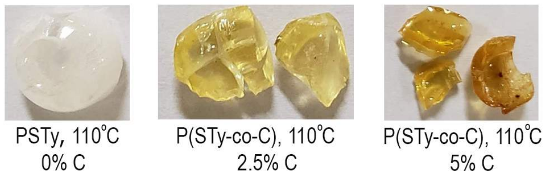
Figure 5.16: Photographs of samples of polystyrene and poly(styrene-co-cardanol) prepared at 110°C
