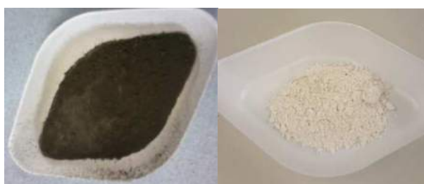
Figure 4.5.3 – 1.2-K/ZrZn/MgO-SiO 2 -(50:50) catalyst after 48 h of reaction use (left) and its image after regeneration (right).
