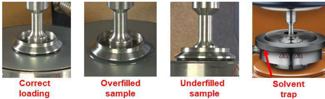
Figure 14 - Three different situations of sample loading of using a parallel plate geometry 40 mm. A schematic representation of solvent trap, used to mitigate solvent evaporation, is also shown.
