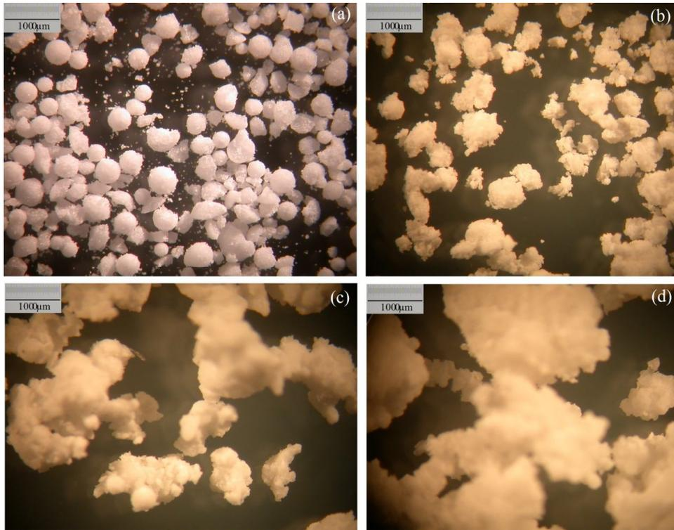
**Figura 4.16:** Micrografia das amostras PPL2(a), PPHDL4 (b), PPHDL5 (c) e PPHDL6 (d).
