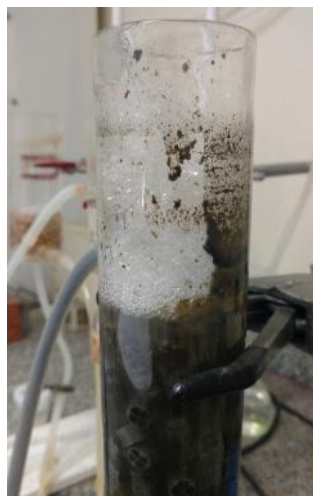
Figure 4.2 – MBBR system showing scum formation during the inadequate IPT dilution (days 100 to 115, Figure 4.1).
