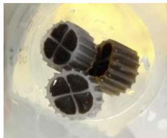
Figure 2.18 – Biofilm carriers (Kaldnes K1) with clogged voids due to poor mixing within the reactor. Source: lab-scale MBBR from pesticide research.
