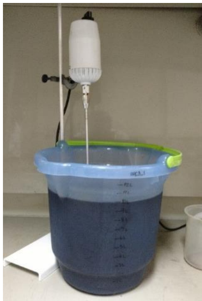
Figure 3.4 – Lab-scale system for reproducing the real scale adsorption onto powdered activated carbon.
