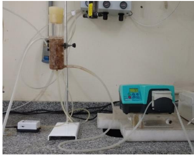
Figure 3.6 – The operating lab-scale MBBR system.
