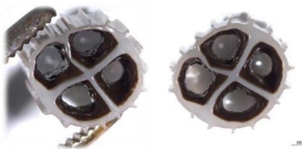
Figure 4.4 – Stereomicroscopy micrographs of the biofilm carriers in phase 7.
